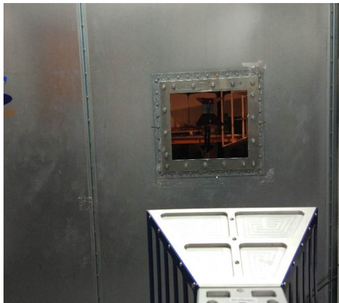
Photograph 7.1.3 Shielding attenuation for electromagnetic and plane waves calibration setup in 1 – 18 GHz range
