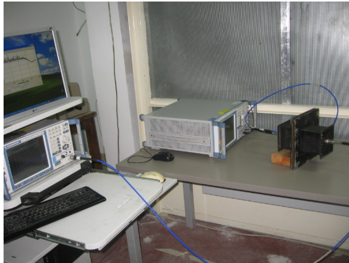
Photograph 7.1.2 Shielding attenuation test setup in 100 kHz – 2 GHz range, electric field
