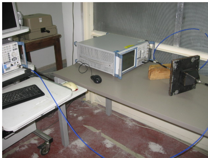
Photograph 7.1.2 Shielding attenuation test setup in 100 kHz – 2 GHz range, electric field
