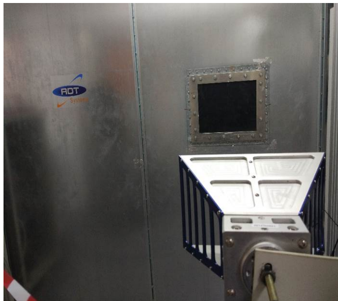
Photograph 7.1.4 Shielding attenuation for electromagnetic and plane waves test setup in 1 – 18 GHz range
